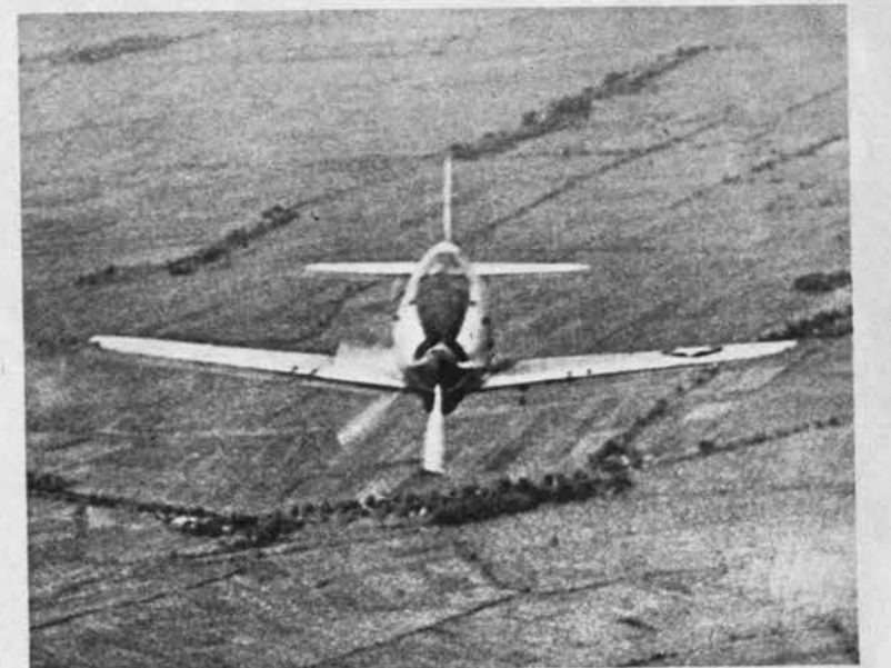
Jack head-on retains bumblebee appearance with short wing and fat round fuselage. Unbroken dihedral is characteristic of most Jap types.
